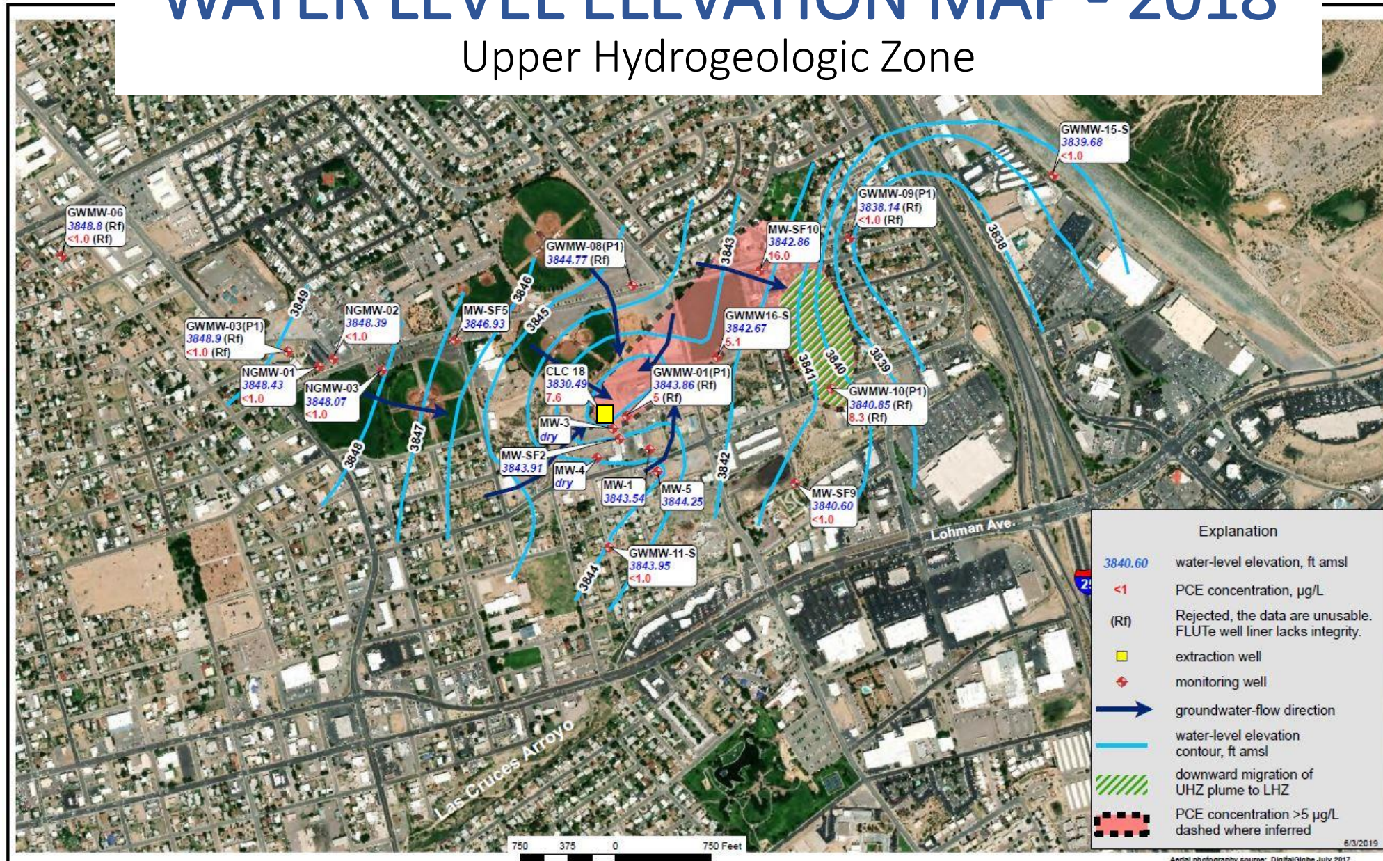
Figure 8. Aerial photograph showing December 2018 water-level elevation contours and PCE concentrations for the Upper Hydrogeologic Zone, Griggs and Walnut Site, Las Cruces, New Mexico.
